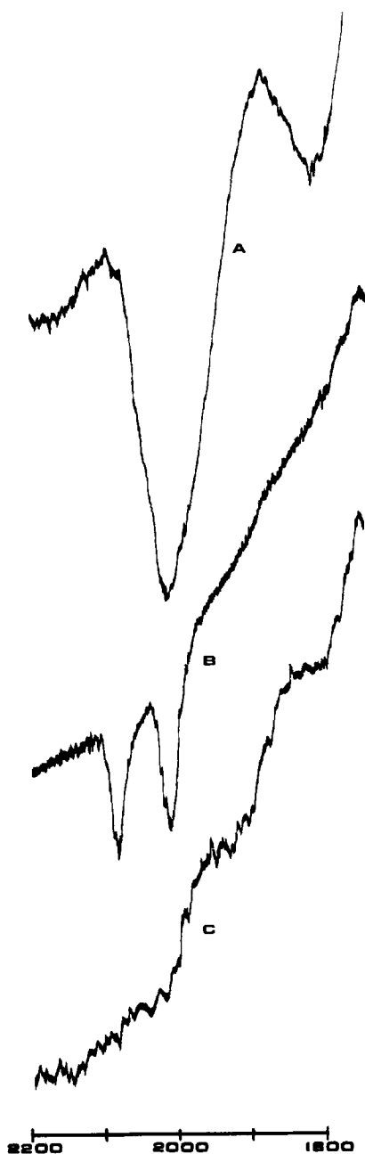
FIG. 9. Ir spectra obtained during oxygenation of a carbonylated sample as represented by gas adsorption plots of Fig. 5. Spectrum (a) is spectrum prior to introduction of O_2 ; spectrum (b) is after 150 hr exposure to O_2 (see Fig. 5); spectrum (c) is for the sample in (b) but after introduction of H_2O at equilibrium vapor pressure.
